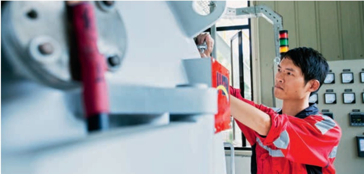
Lab furnace for CAB brazing at Gränges Application centre in Shanghai.
