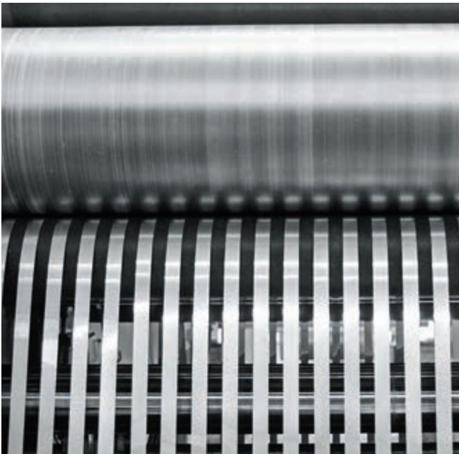
Slitting machine in the production flow and slit aluminium strips for clad fin.
