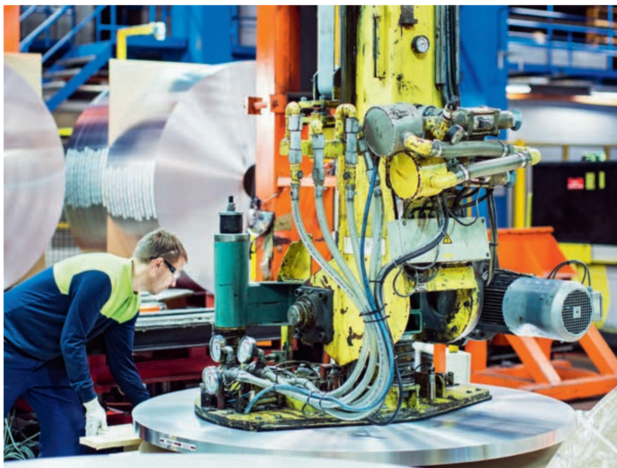
Vacuum lift for aluminium strips in finishing before shipment from Gränges in Finspång.
